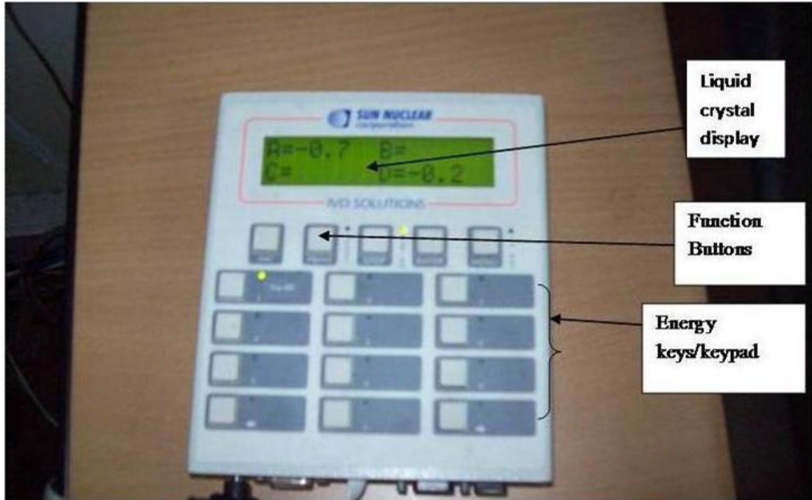
Figure 2. Control Panel and display screen of the diodes.
