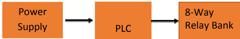
Figure 3. Block diagram of the PTS control unit
